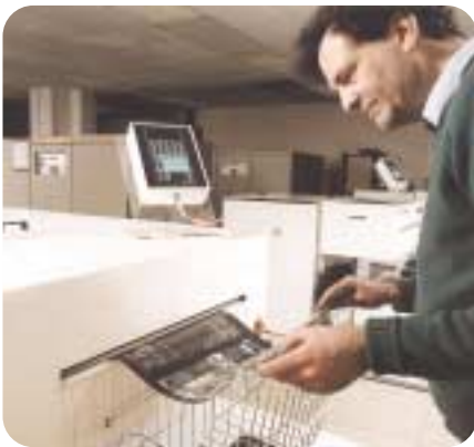
Conventional printing requires an imagesetter to create the films which are then used to create plates.
