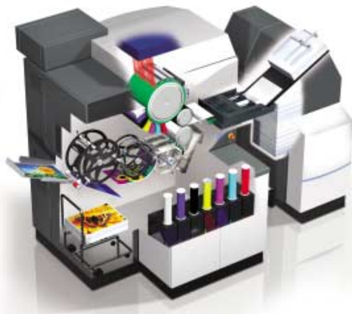
A cross section of the HP Indigo Press 3000
